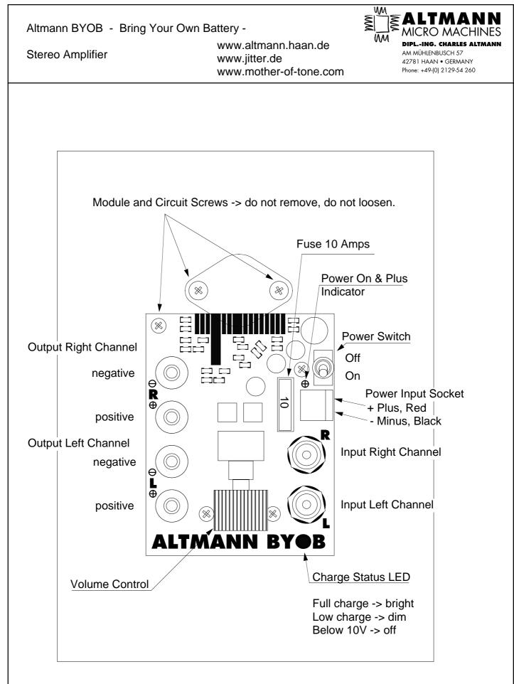
Check polarity before connecting to battery.
